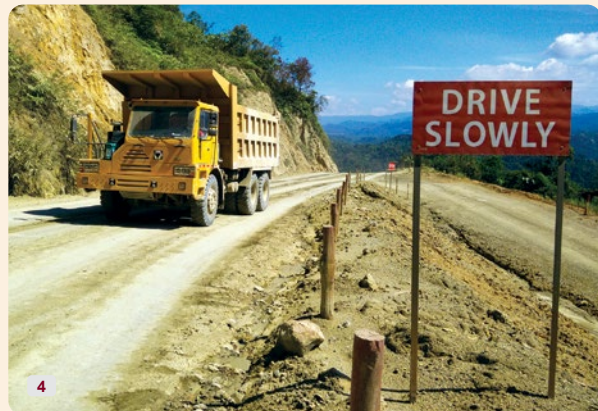
4 Dump truck carrying tailings
