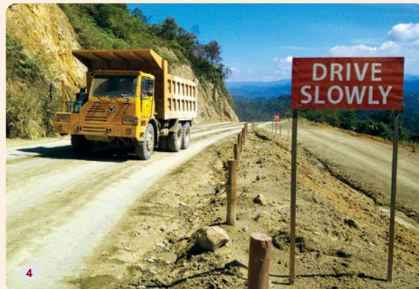
4 Dump truck carrying tailings
